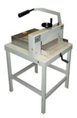
This heavy duty stack cutter has a maximum cutting capacity of 800 sheets of 20lb paper. Cutting width up to 18". Features hand clamp and back gauge and measuring scale in inches and millimeters. Safety features include protective shield on both sides of blade and cutting guard activated safety lock.
