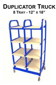
For all 11" x 17" printing presses. The portable drying/ storage rack has eight 12" x 18" removable shelves. This allows printed material to be transferred from press to rack without being touched by hands. Rolls easily, even when filled to capacity. Rugged construction of welded square tube steel. Heavy-duty casters, two with brakes for stability. Overall size, 28" wide, 18" deep, and 48" high. Shipping weight 110 lb.
