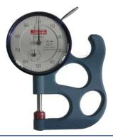
Designed to accurately measure paper, laminates and plates. Dial face is 2 5/8" in diameter. Lever activated measurement accurate up to 0.001" Measuring capacity is .5 inches.
