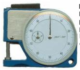
Easily held in natural grip. Ideal for measurement of plates, packing materials, paper, blankets or wire. Fraction and decimal equivalents on back of case. Dial diameter is 1 7/8". Accuracy is up to 0.001". Measuring capacity is .5 inches.
