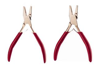
Cuts and crimps coil sizes from 5 mm to 33 mm. Recommended for use with coil inserters that do not have automatic crimping. Red dot facing upward indicates the proper position for crimping. Longer crimp length prevents coil from unwinding out of book.
